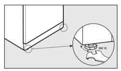
Align the feet using the spanner supplied.
